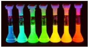
Figure 2. CdSe QDs of different sizes can fine-tune optical absorption properties.
