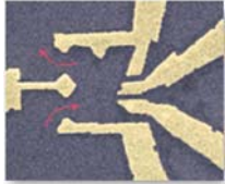
Fig. 1. In this case, electrons are confined vertically due to the interface between GaAs/AlGaAs, metallic gates confine the electrons laterally.
