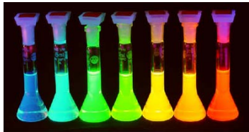
Fig. 2. Fluorescence induced by exposure to ultraviolet light in vials containing various sized Cadmium Selenide (CdSe) quantum dots.
